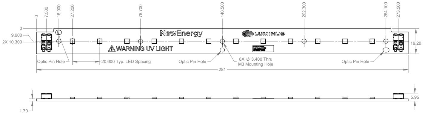
1. Two Position Poke-In Connectors accept 18-24 AWG solid or stranded wire
