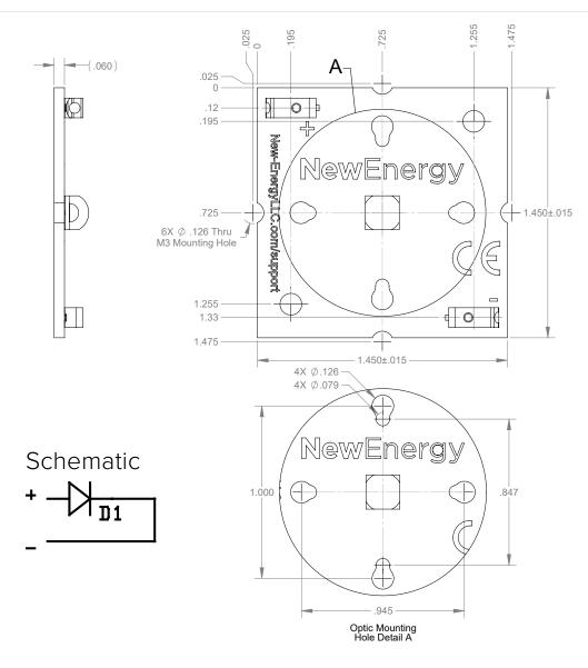
1. Single Poke-In Connectors accept 22-26 AWG solid or stranded wire
