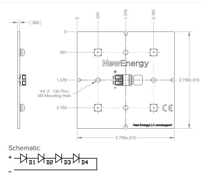
1. Dual Poke-In Connectors accept 18-24 AWG solid or stranded wire
